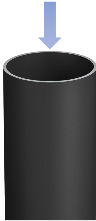
The tube wall thickness is 1.2 mm.
